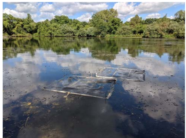
Fig. 4. Mesocosm racks floating in a pond at Hanley Preserve. Incubations were conducted in a small pond at the HWS Hanley Preserve to reduce the likelihood of losing or breaking a rack due to waves and winds in Owasco Lake. Temperature and solar radiation measurements were made at the site every five minutes during the seven day incubation.
